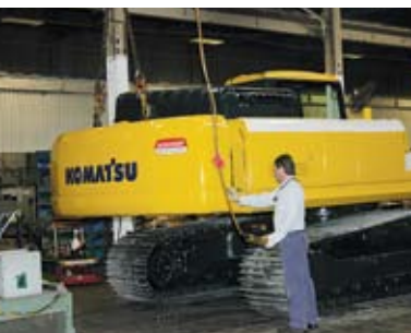
Using an overhead crane, a worker installs the counterweight on a PC300LC-7 at the Chattanooga plant.
