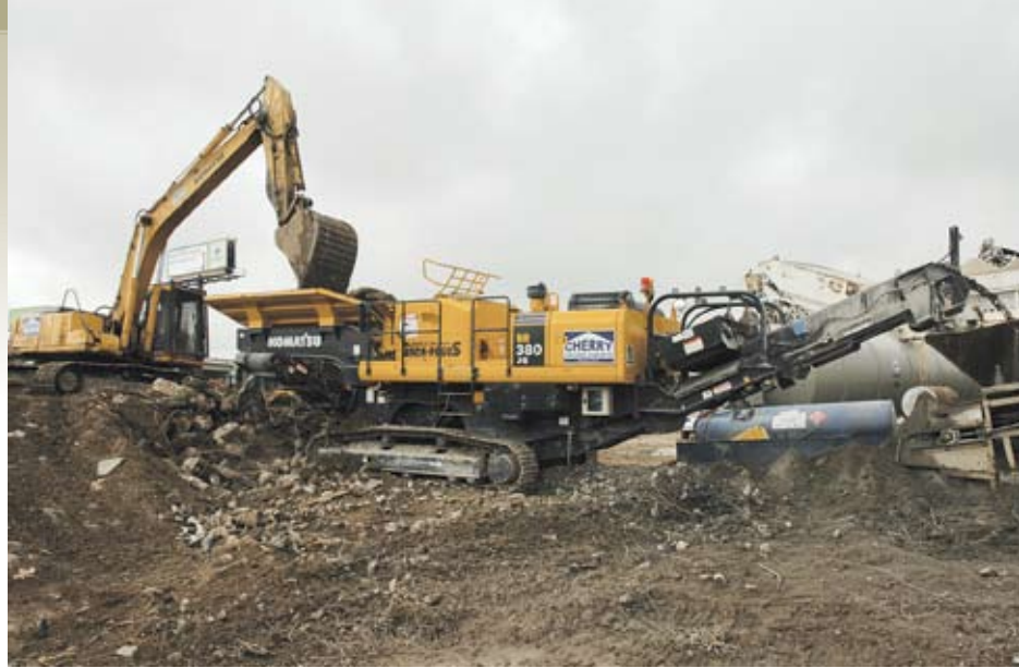
A Cherry Portable Crushing operator uses a Komatsu PC220 excavator to load material into a Komatsu BR380JG crusher at a project in Beaumont. "On an average day we're producing 600 to 800 tons of five-inch-minus product with the BR380," said General Manager Wesley Guidry. "That's good production, and we expect it to continue to go up as our experience grows."
