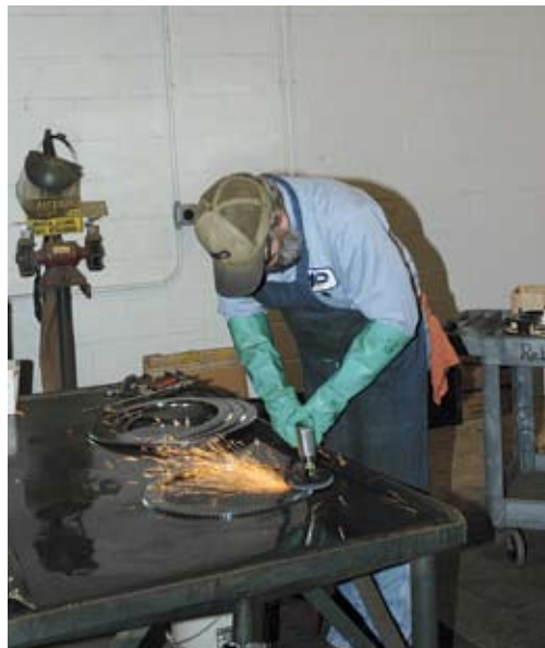
Making sure components are free of dirt and contaminants takes several steps, including grinding.
