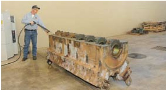
The first step in the remanufacturing process is a thorough cleaning, such as the one Paul Dillon gives to this engine block in the wash bay located behind the new building.
