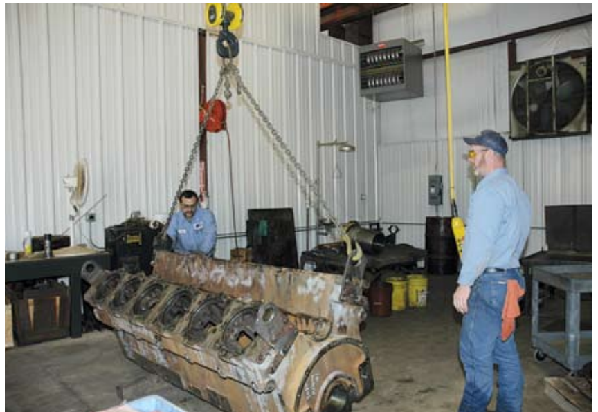
After washing down the component outside, a WPI reman specialist brings it into a cleaning room and makes it virtually spotless with cleaning agents, such as solvents.
