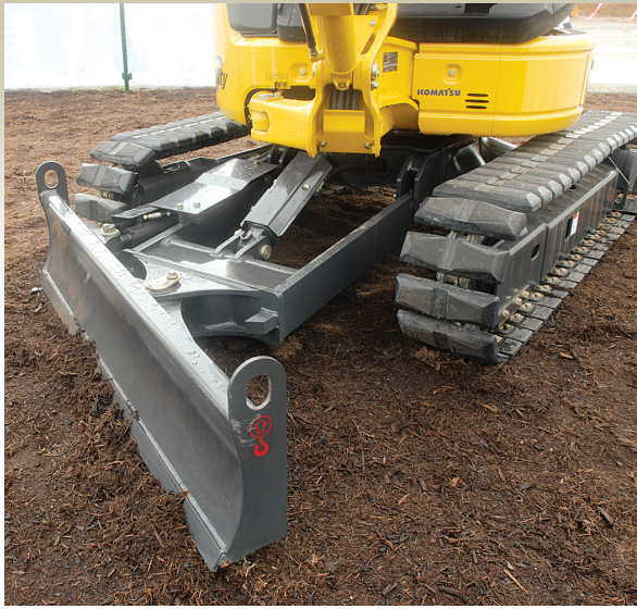
David Caldwell, Product Manager for Compact Excavators, shows attendees some of the benefits of Komatsu excavators, such as the tilt-up canopy and four-way blade (shown above) on the PC50MR-2.
