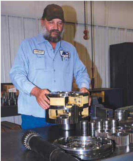
Technician James Terry works with a disassembled Komatsu HD785 transmission that will be rebuilt. WPI's Kilgore remanufacturing facility rebuilds mining components back to OEM specs using OEM parts, and offers a full, one-year warranty.
