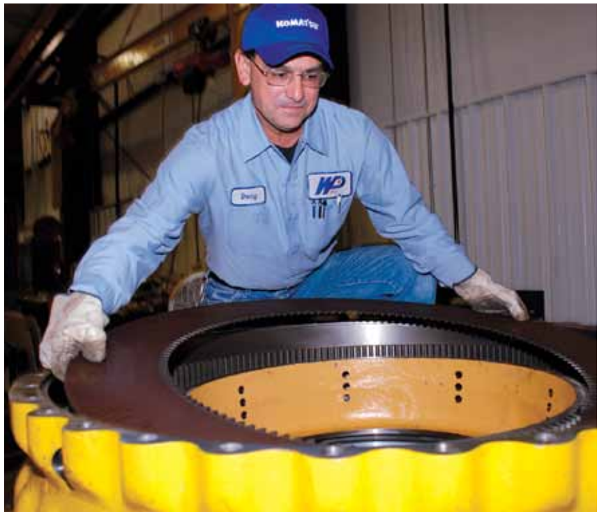
Technician Donny Lopez installs a disc on a rear brake assembly for a Komatsu HD1500 haul truck.
