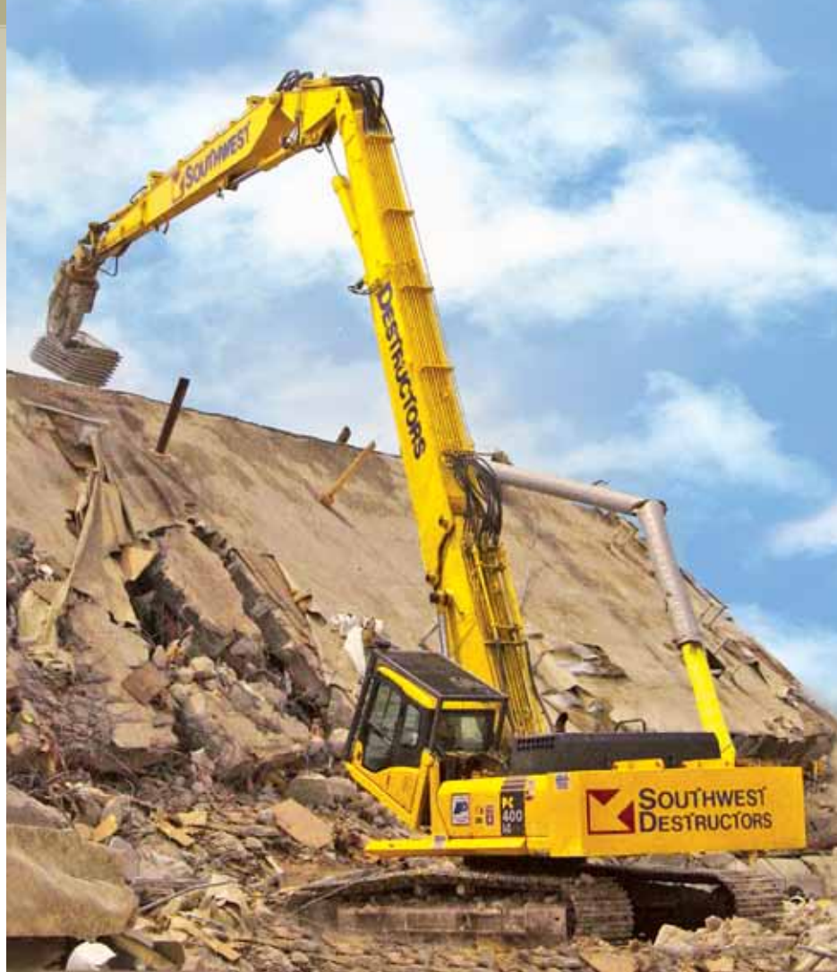
Southwest Destructors uses a wide range of Komatsu excavators, including this PC400LC-8 high-reach for larger buildings. “I believe to be efficient, we have to have the right tool for the job, and the PC400 high-reach is the proper tool for larger structures,” said Vice President Ross Rathgeber.
