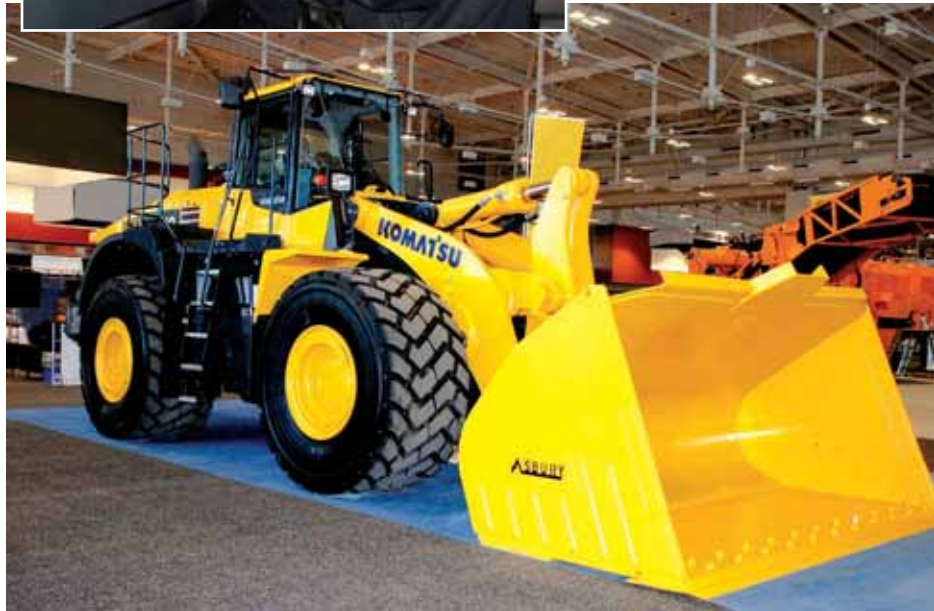
Attendees of the 2016 Asphalt Show & Conference and AGG1 Academy & Expo check out the Komatsu WA500-7 Yard Loader arrangement. The 79,000-pound-plus loader that Komatsu displayed features a 9.8-cubic-yard, flat-floor bucket, which increases capacity and productivity for applications involving re-handled or loose materials.
