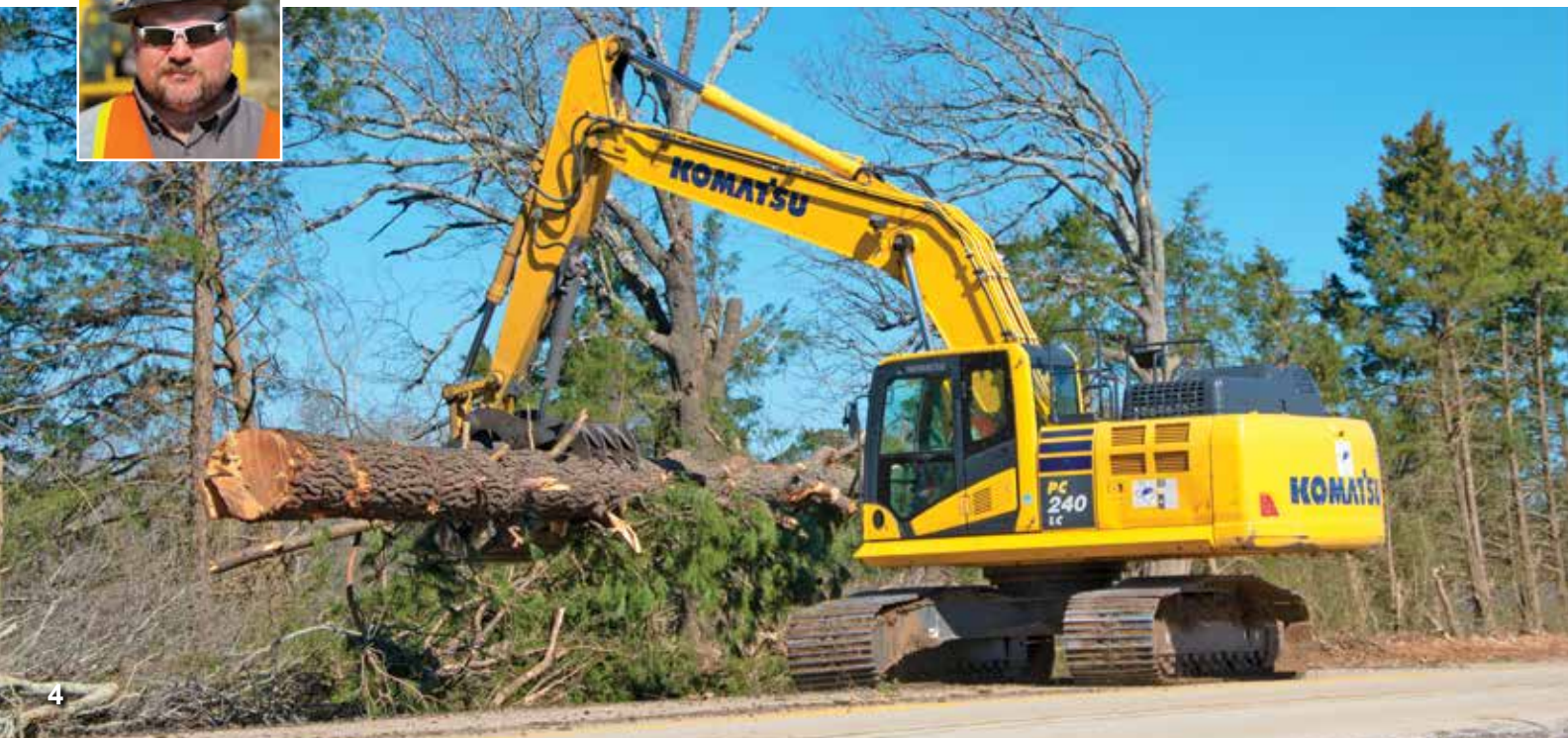
Foreman Brent Oliver moves timber with a Komatsu PC240LC-11 excavator equipped with a grapple. "We have three Komatsu excavators of varying sizes, and we match them to the task," said Oliver. "They all have good power, and the production is outstanding."
