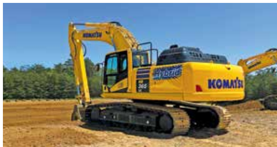
Komatsu's HB365LC-3 hybrid excavator delivers eco-conscious performance as energy is captured during swing and stored in the ultracapacitor.
