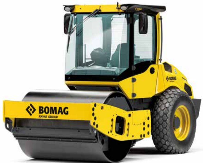
BOMAG's BW 177 BVO-5 PL single drum roller features three compaction modes, making it ideal for a range of soil applications on small and medium construction sites.
